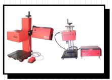
EtchON DPM301/301D ", This is a perfect startup Pneumatic PC based Dot Pin Marking Machine suitable for small and light work piece support plain as well as arc marking. Marking head adopted the highest quality imported linear guide with Auto Lubrication (Export Series)
